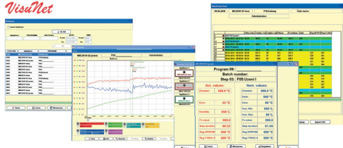
The VisuNet system enables data evidence and a remote access to the chamber control from your PC.
